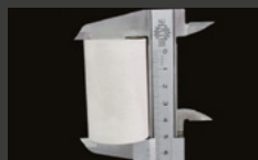
Carefully level the ring so that the top and bottom are perpendicular to the sides of the ring
