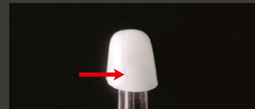
Crack is happened during grinding
