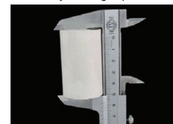
Carefully level the ring so that the top and bottom are perpendicular to the sides of the ring.
