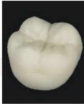
Ceramic crown after press-molding
